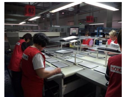
Fig.3 Placing the cover parts in the thermos-tunnel to activate the laminating adhesive
